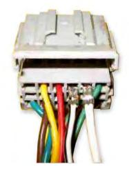
5. Wrap the connector with foam tape (EPT sealer 3T), and reconnect the harness.
